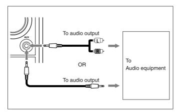
When the audio equipment has pin jacks for audio output: Be sure that the pin plugs of the audio cords are colored—white plugs and jacks are for left audio signals, and red ones for right audio signals.
